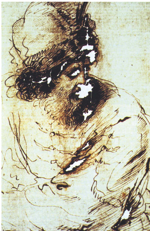
Figure 7 Iron-gall ink burn on a Guercino (1599–1666) drawing. The holes are the result of iron-catalysed degradation and acid-catalysed hydrolysis.
